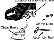
An adjusting pin and screw is used to adjust the tension of the chain. It is very important when assembling the bar, that the pin located on the adjusting screw aligns into a hole in the bar. Turning the screw will move the adjustment pin up and down the screw. Locate this adjustment before you begin mounting the bar onto the saw.
